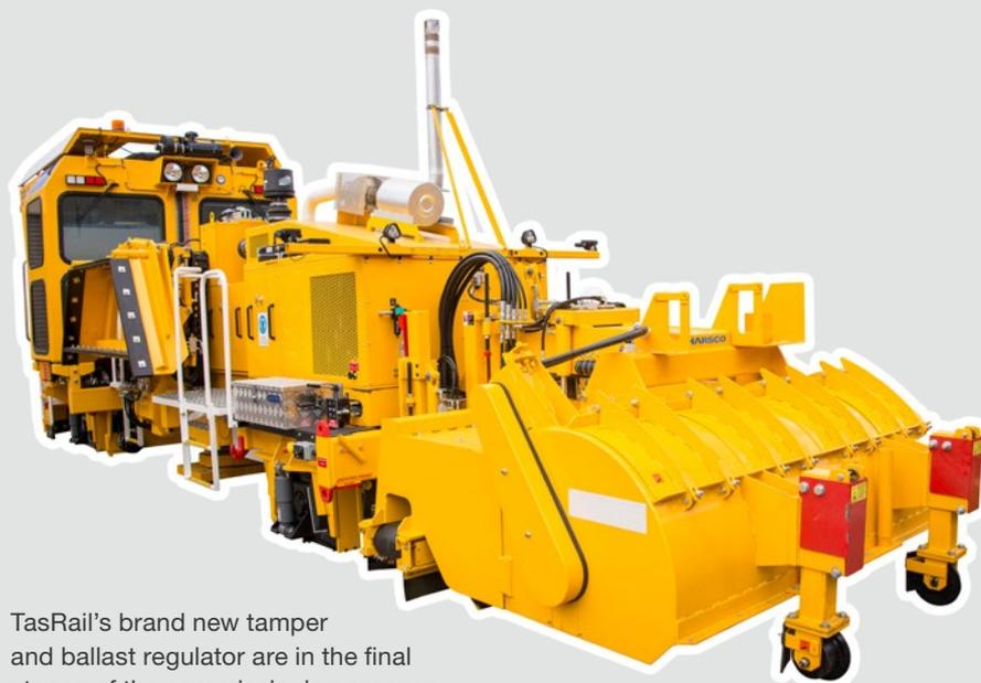
TasRail's brand new tamper and ballast regulator are in the final stages of the commissioning process.
